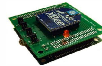
Missouri S&T Mote, RFID tag for networking sensing and decentralized control, diagnostics and prognostics
